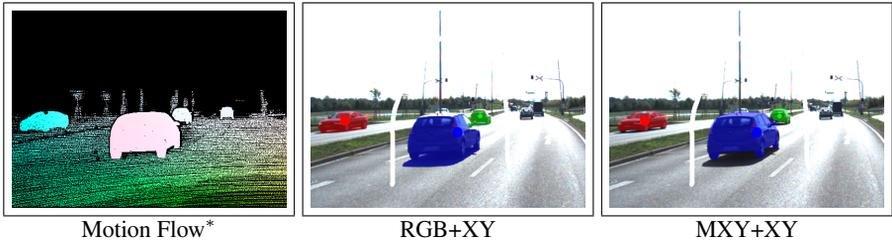
Fig. 9: Kernel cut on image 000079\_10 from *KITTI* [43]. The images show the motion flow, color-based segmentation (RGB+XY), motion based segmentation with location features (MX+XY). \* Black color shows pixels that lack motion information.
