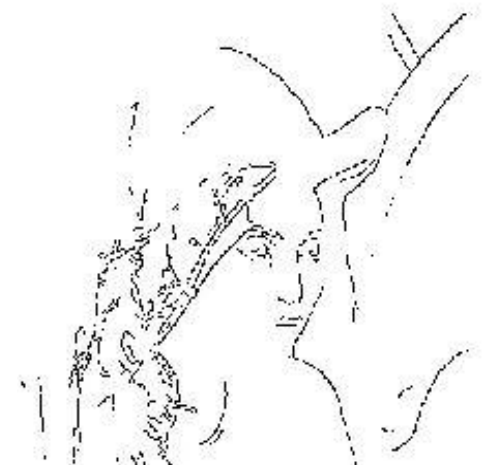
Canny edge detector (non-maxima suppression + adaptive thresholding)
