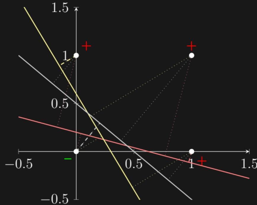
$$\max_{\mathbf{w}: \forall i, y_i \hat{y}_i > 0} \min_{i=1, \dots, n} \frac{y_i \hat{y}_i}{\|\mathbf{w}\|}, \quad \text{where} \quad \hat{y}_i := \langle \mathbf{x}_i, \mathbf{w} \rangle + b$$
