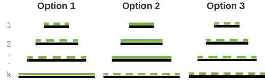
Figure 4: Possible options at k -th step of MinEnt algorithm. Option 1 distributes as much slack as possible to \hat{p}_k (solid green line) and the rest to \hat{p}_1, \dots, \hat{p}_{k-1} (dotted green line). Option 2 distributes as much slack as possible to \hat{p}_1, \dots, \hat{p}_{k-1} and the rest to \hat{p}_k . Option 3 distributes slack to \hat{p}_1, \dots, \hat{p}_{k-1} and \hat{p}_k instead of distributing as much as possible to either.
