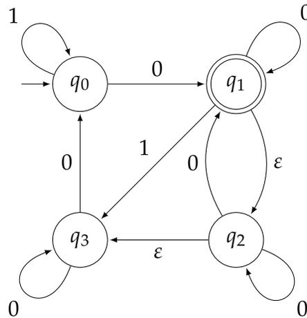
Figure 3.1: The state diagram of an NFA.
