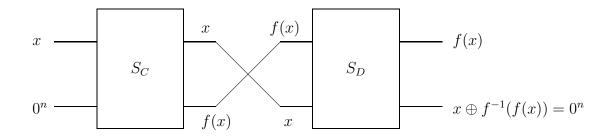
(In order to simplify the picture, each "wire" represents n bits and the ancilla bits needed by the circuits  $S_C$  and  $S_D$  have not been shown explicitly.)
