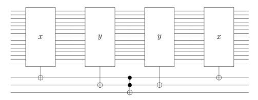
Of course this requires communication: they must exchange  $O(\log n)$  qubits in order to implement this circuit. However, that is good enough for what we need: Alice (say) can effectively run Grover's Algorithm to determine whether  $x_i \wedge y_i = 1$  for some *i*, exchanging  $O(\log n)$  qubits with Bob for each query. Because the total number of queries needed is at most  $O(\sqrt{n})$ , the total amount of communication is  $O(\sqrt{n} \log n)$ .
