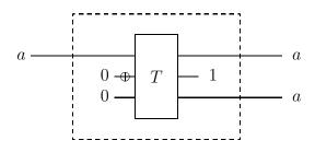
Of course it would have been just as easy to input a 1 into the second input of the Toffoli gate rather than performing a NOT operation on a 0. I've only written it like this because it will be convenient later to have all of the auxiliary inputs start in the 0 state.
