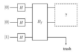
Let us analyze the state of the above circuit at various instants to try and determine what (if anything) would work for the omitted part of the circuit. The state after the Hadamard transforms can be written
