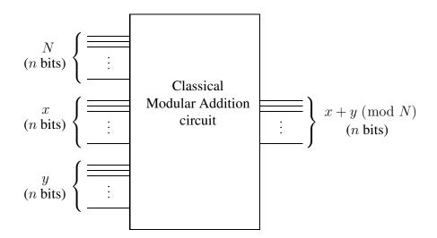
Obviously such a circuit is non-unitary—the number of input and output qubits do not even agree. If we are to somehow transform this circuit into a valid quantum circuit, it will have to correspond to a unitary transformation.
