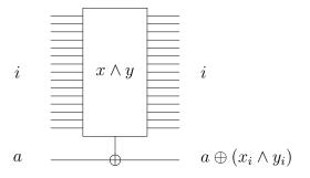
Using  $O(\sqrt{n})$  queries to this black box, Grover's Algorithm could determine with high probability whether there exists an index *i* for which g(i) = 1 (which is equivalent to  $x_i \wedge y_i = 1$ ).
