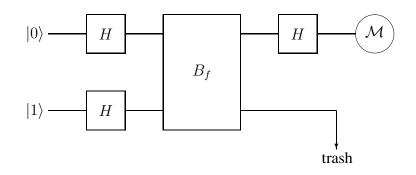
This procedure is known as *Deutsch's Algorithm*, and the problem of determining whether a one-bit function is constant or balanced is sometimes called *Deutsch's Problem*.
