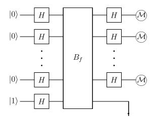
There are n bits resulting from the measurements. If all n measurement results are 0, we conclude that the function was constant. Otherwise, if at least one of the measurement outcomes is 1, we conclude that the function was balanced.
