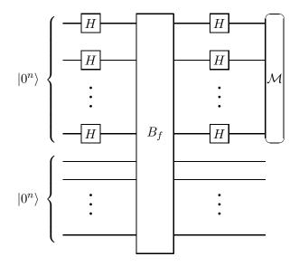
Note that the  $B_f$  gate has a different (but very similar) form from before because the input and output of the function f are n-bit strings:
