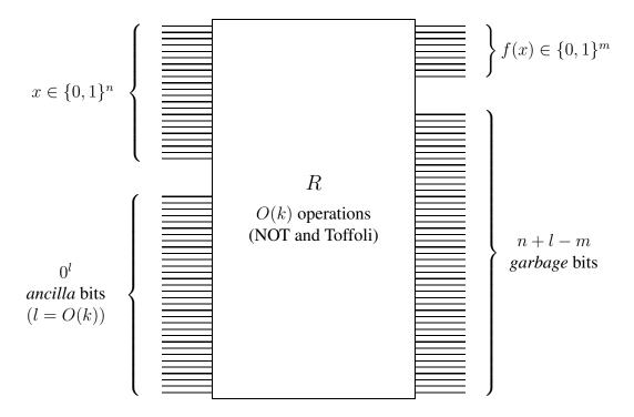
The auxiliary bits needed for the AND and FANOUT simulations in this circuit are sometimes called *ancilla* bits. The bits labeled *garbage* are the extra bits that resulted from the simulations (that were left inside the dashed boxes in the above pictures).
