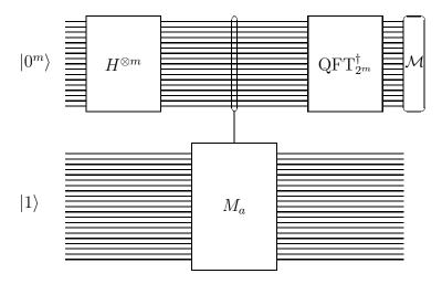
(It can be run sequentially several times to improve accuracy.) Plug the measurement outcome  $j/2^m$  along with N into the continued fraction algorithm, which gives a fraction x/y. Repeat the entire process several times, taking the least common multiple of the y values. The result will be r with high probability. The entire process is known as Shor's algorithm for order finding.
