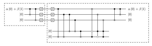
As you would expect, although the new code protects against phase-flips, it fails to protect against bit-flips (and in fact makes matters worse for bit-flips just as happened previously for phase-flips).
