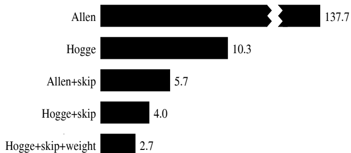
Figure 5: Effect of heuristics on time (sec.) of path consistency algorithms applied to Benzer's matrix
