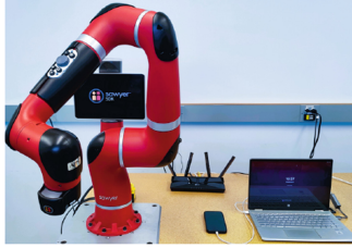
Fig. 1. The smartphone sends signals to the robot control software on a computer via cable, and the computer communicates with the robot over the same network.
