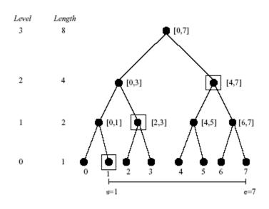
Range [1-7] broken down into 3 sub-ranges
