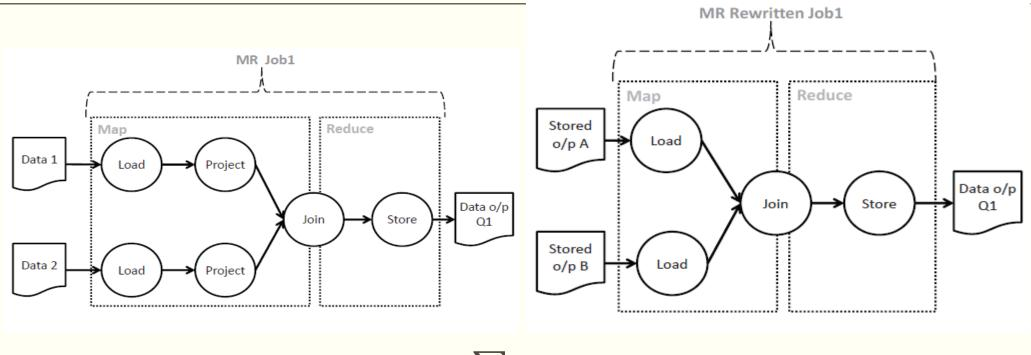
$$ET(Job_n) = T_{load} + \sum_i ET(OP_i) + T_{sort} + T_{store}$$
