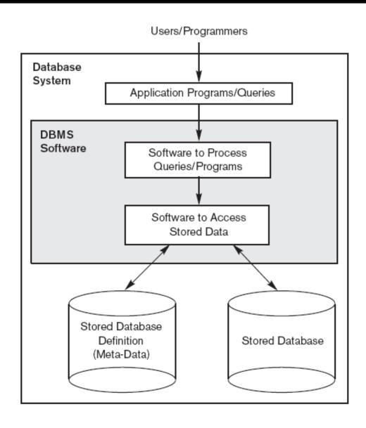
Figure 1.1 A simplified database system environment.
