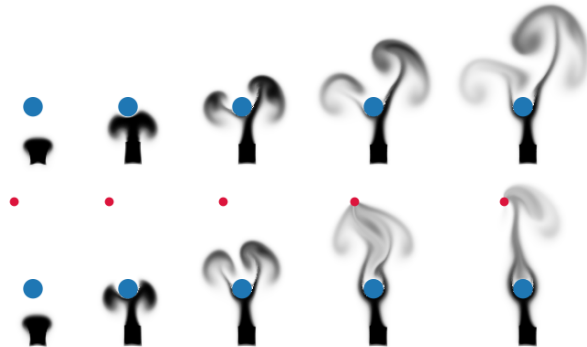
Figure 4: Buoyancy and divergence control (resolution 256^2 ). We simulate a hot smoke plume rising towards a blue circular obstacle in 2D using the Boussinesq buoyancy model (left). We can also add a velocity sink to the scene, indicated with a red dot, causing the smoke to be sucked into the sink (right). ● 3m49s
