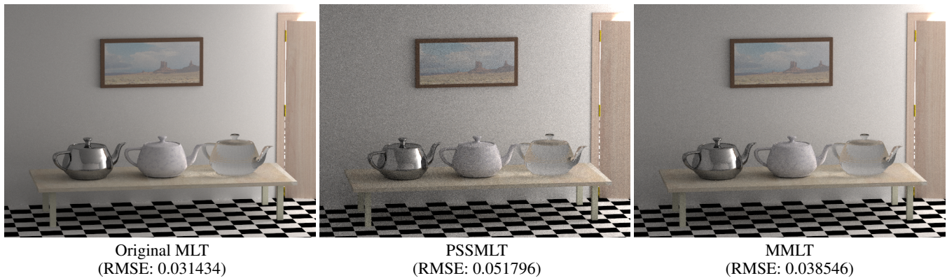
Figure 9: Comparison of original MLT (left), primary sample space MLT (center), and multiplexed MLT (right) for the door scene without glossy materials (90 min). Original MLT works quite well in this scene since their mutation strategies are well suited to handle paths with Lambertian and specular materials. While multiplexed MLT is slightly outperformed by original MLT, it still improves upon primary sample space by automatically distribute samples across different techniques according to their weighted contributions.
