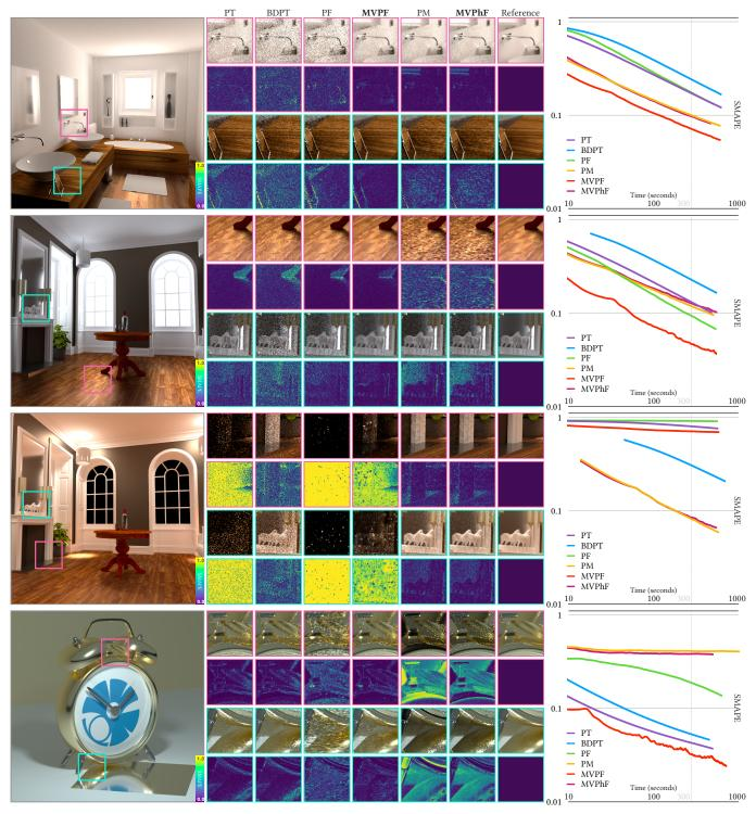
Fig. 1. An equal-time comparison of path tracing (PT), bidirectional path tracing (BDPT), single vertex path filtering (PF), photon mapping (PM), multi-vertex path filtering (MVPF), and multi-vertex photon filtering (MVPhF) on four additional scenes that cover various real-world lighting scenarios.
