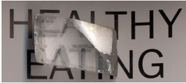
Figure 13: Birefringence of calcite (©Wikipedia). Note that even this photograph take at right angle to the surface of calcite, there is birefringence caused by ordinary ray and extraordinary ray.
