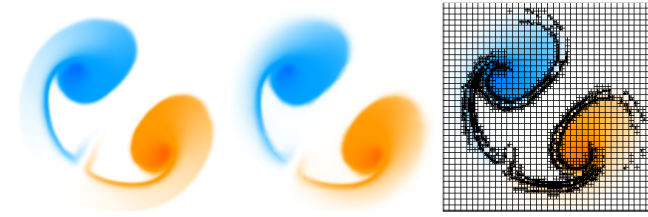
Fig. 16. Fluid simulation results using a uniform cache (left) and an adaptive cache (middle) using one-twentieth memory footprint that of the uniform one. Slowly varying regions are sparsely cached while dense sampling occurs in regions exhibiting steep or discontinuous variations.
