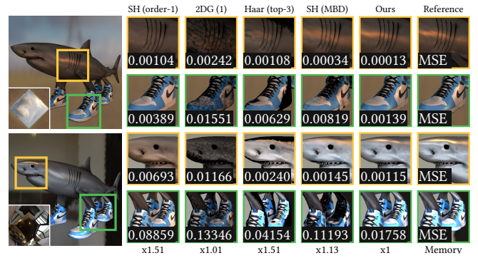
Fig. 18. GLOSSY GLOBAL ILLUMINATION. We approximate glossy transport with multiple bounces under a fixed camera view. Under an equal memory budget, our method outperforms baseline approaches in reproducing specular highlights across different environment maps.
