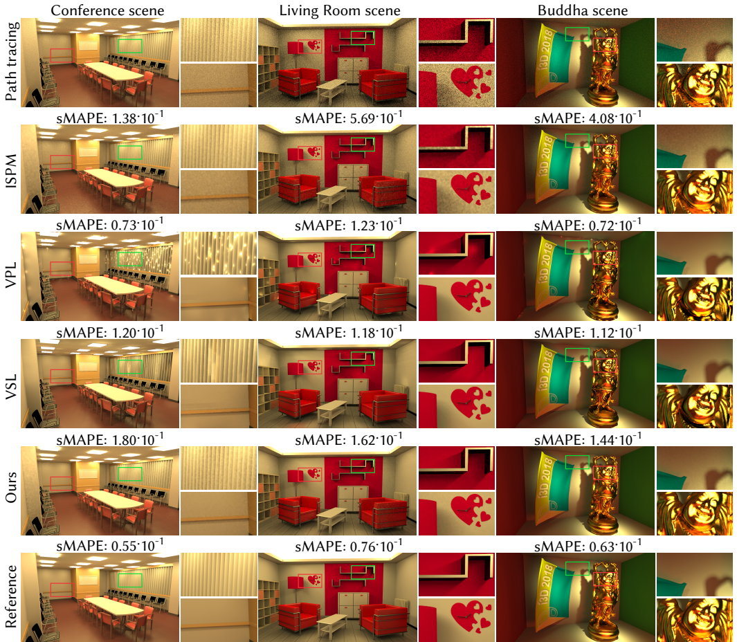
Fig. 6. Equal-time comparisons in 15 seconds between GPU path tracing, image space photon mapping (ISPM) [McGuire and Luebke 2009], virtual point light (VPL) [Keller 1997], virtual spherical light (VSL) [Hašan et al. 2009], and our method. Path tracing and ISPM usually exhibit a visible level of noise. In comparison, VPL produces smoother images but suffers from the singularities. VSL solves this problem but introduces a visible level of bias. Our method provides results close to the reference.
