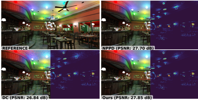
Figure 4: Comparison of our method with the NPPD and DC baselines on the Bistro3 [Lum17] scene at 8 spp. Our approach (w/pyramid) reduces errors around the light source by leveraging path-tracing inputs. Unlike DC, which tends to introduce artifacts under low-spp conditions, our generalized fusion of multiple correlated inputs effectively suppresses such artifacts.
