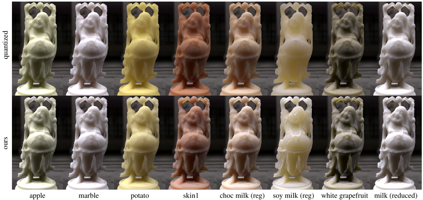
Fig. 11. Image based lighting of the Happy Buddha model with the materials also used in the simple test cases (Figure 7). The images were rendered using hierarchical integration of the quantized diffusion model [d’Eon and Irving 2011] plus single scattering added by separate Monte Carlo ray tracing (top row) and our model (bottom row). We excluded Fresnel reflection in order to better highlight the differences between the two models.
