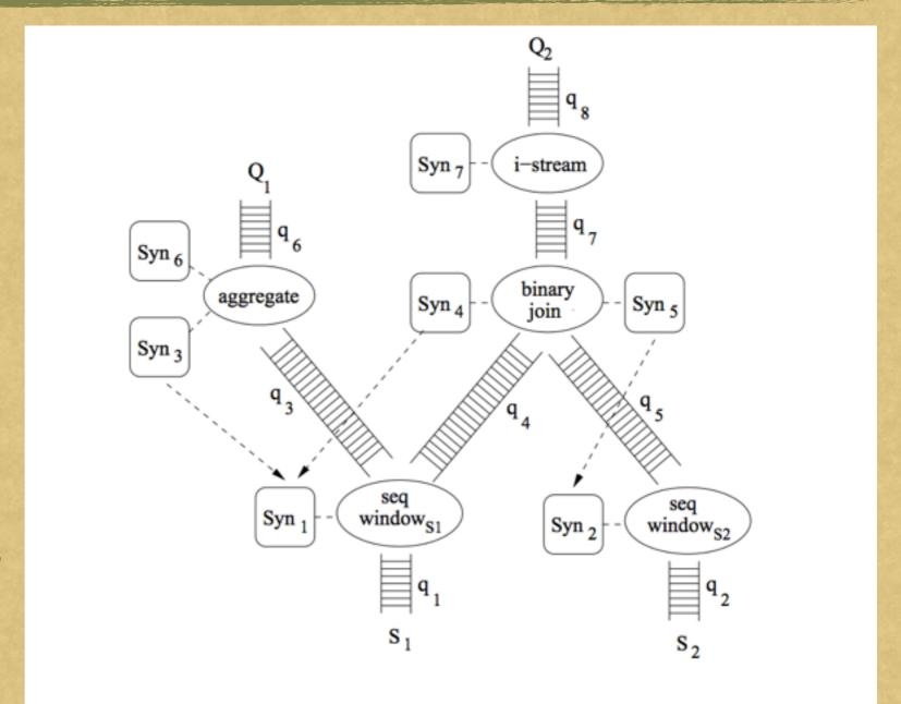
Figure 4: STREAM continuous query plan for two queries
