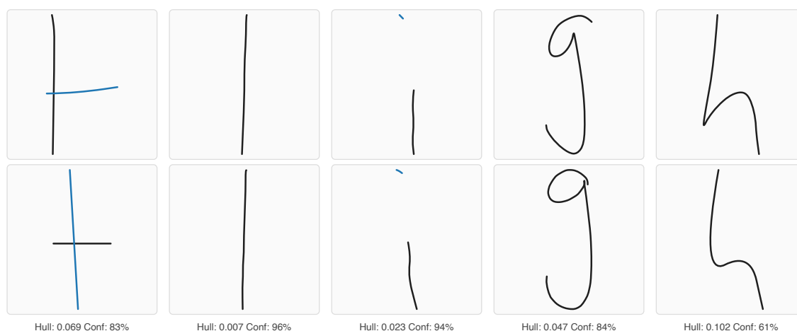
Figure 8.1: High → tligh . Trace-grouping over-segmentation: the capital H is split into a t and an l by a within-character gap.
