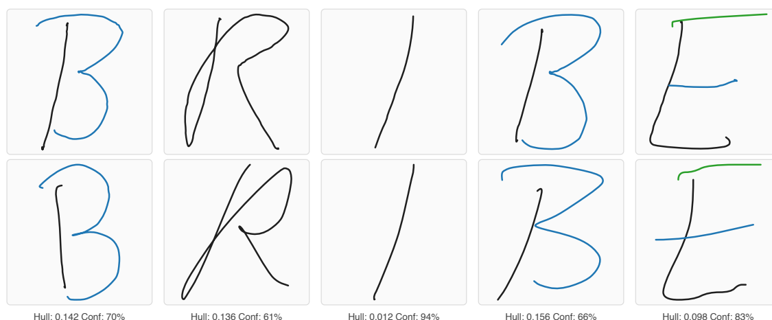
Figure 8.3: BRIBE \rightarrow BRlBE. Superclass-equivalent recognition error: the capital I written as a plain vertical pen mark is matched against an equally plain vertical pen mark from the lowercase-l class.
