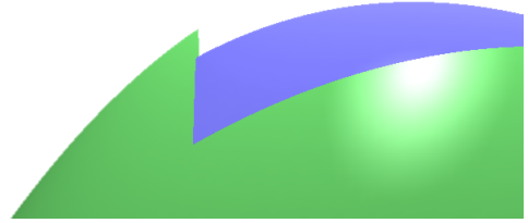
Figure 2: C^0 discontinuity in standard surface pasting
