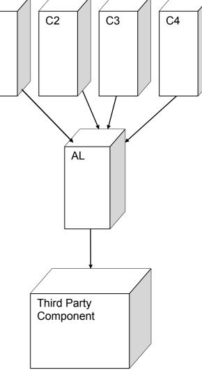
Only the AL (abstraction layer) component is directly dependent on the third party component. If the third party component is replaced, changes are restricted to the AL component only
