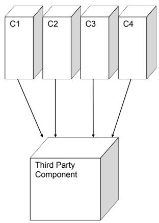
Four components are directly dependent on a third party component. If the third party component is replaced with a new component with a different interface, changes to each component are likely.
