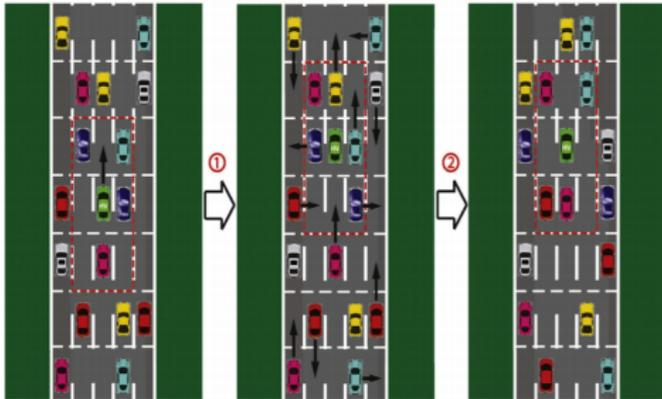
The above graphic shows one transition cycle, where the HV selects the "accelerate" action and the surrounding vehicle subsequently select their actions. The HV selects their action based only on the surrounding vehicles, denoted by the red grid.
