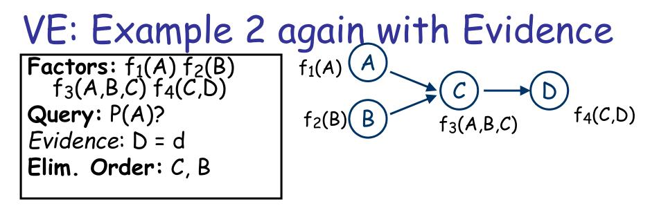
Restriction: replace  $f_4(C,D)$  with  $f_5(C) = f_4(C,d)$ Step 1: Add  $f_6(A,B) = \sum_C f_5(C) f_3(A,B,C)$ Remove:  $f_3(A,B,C), f_5(C)$ Step 2: Add  $f_7(A) = \sum_B f_6(A,B) f_2(B)$ Remove:  $f_6(A,B), f_2(B)$ Last factors:  $f_7(A), f_1(A)$ . The product  $f_1(A) \times f_7(A)$  is (possibly unnormalized) posterior. So...  $P(A|d) = \alpha f_1(A) \times f_7(A)$ .
