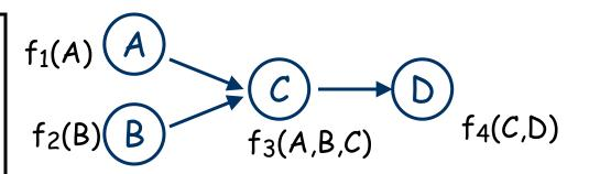
Step 1: Add  $f_5(B,C) = \Sigma_A f_3(A,B,C) f_1(A)$
