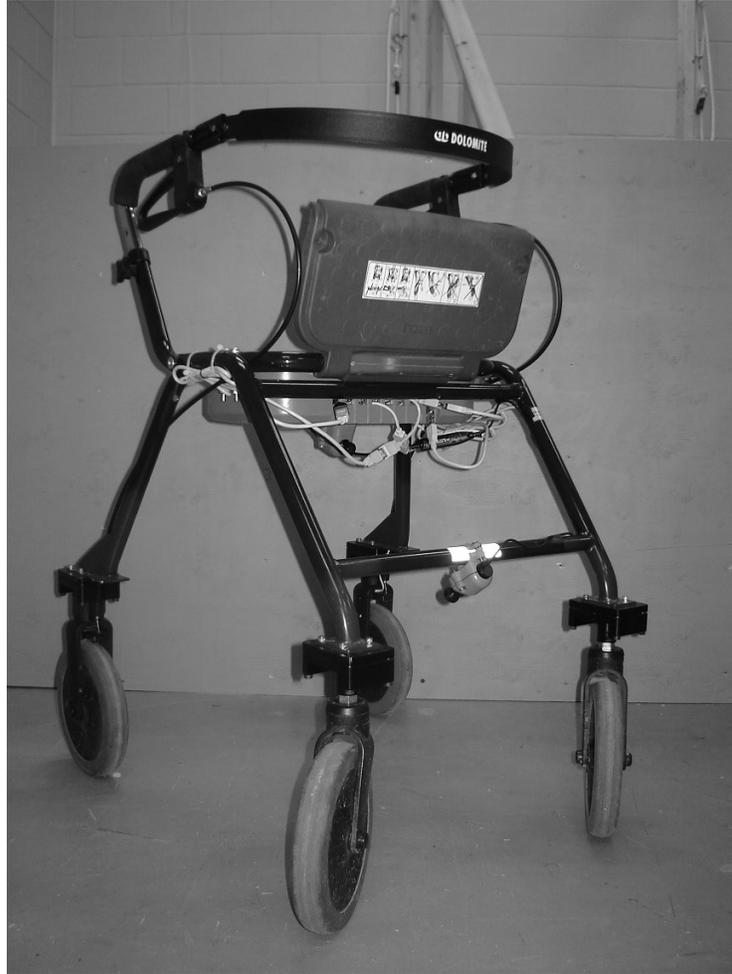
Figure 1.1: The instrumented walker developed by [73] et. al. The walker has a 3-D accelerometer, 4 load cells, 1 wheel encoder and 2 cameras
