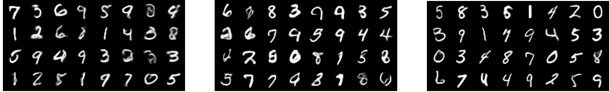
Figure 1: Left: Generated MNIST images with \beta = 0.05 in Eq. 2. Middle: Generated MNIST images with \beta = 1.0 in Eq. 2. Right: Reconstructed MNIST images with \beta = 1.0 in Eq. 2.
