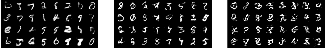
Figure 5: Variation in bottleneck width causes massive differences in generative quality without regularization. From left to right, we present samples ( from \mathcal{N}(0, I) for 8, 16, 32 dimensional latent spaces )
