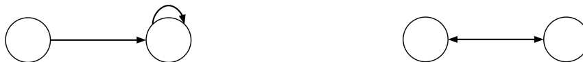
Figure 2.4: Multiple instances of a transition system for the constraint: “every state must reach a state that is reachable from itself” (figure from [42])
