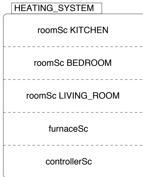
Figure 4.7: Heating system top-level specification
