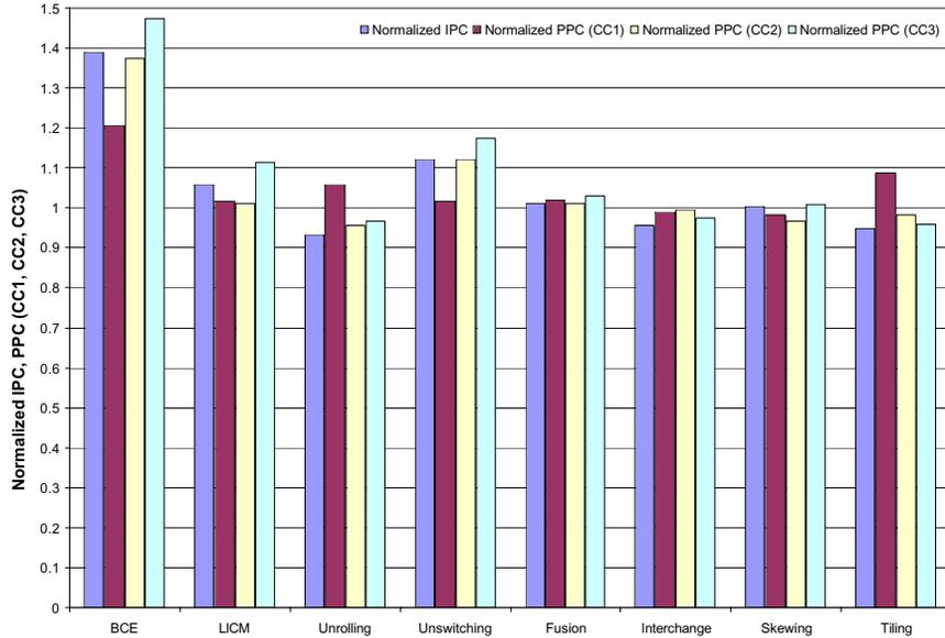
**Figure 4: A comparison of the change in instructions per cycle, to the change in power consumed per cycle measured by the CC1, CC2, and CC3 power models for loop optimizations.**
