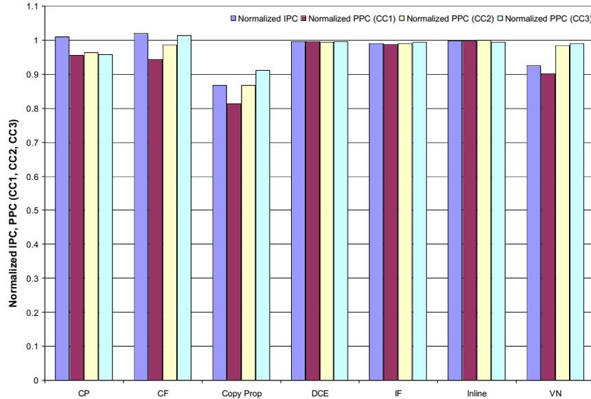
Figure 3: A comparison of the change in instructions per cycle, to the change in power consumed per cycle measured by the CC1, CC2, and CC3 power models for early optimizations.
