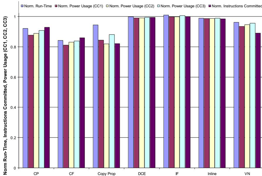
Figure 1: A comparison of the normalized execution time (optimized version divided by baseline version), the normalized power consumption (CC1, CC2, and CC3), and the normalized number of instructions committed as a result of applying each of the early optimizations.
