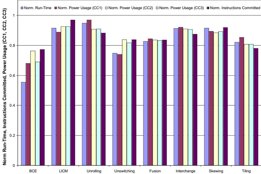
**Figure 2: A comparison of the normalized execution time, the normalized power consumption (CC1,CC2, and CC3), and the normalized number of instructions committed as a result of applying each of the loop optimizations.**
