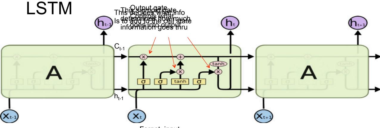
The core idea is this cell state  $C_t$ , it is changed slowly, with only minor linear interactions. It is very easy for information to flow along it unchanged.
