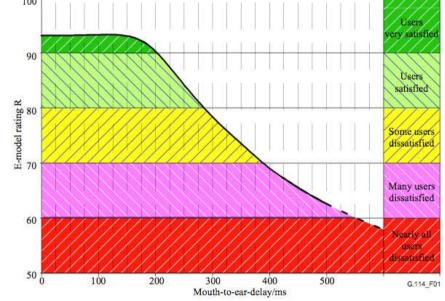
Figure 1/G.114 - Determination of the effects of absolute delay by the E-model
