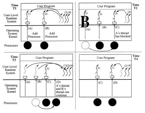
Fig. 1. Example: I/O request/completion.
