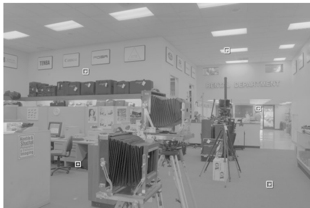
Figure 5: The reconstructed high dynamic range radiance map, mapped into a grayscale image by taking the logarithm of the radiance values. The relative radiance values of the marked pixel locations, clockwise from lower left: 1.0, 46.2, 1907.1, 15116.0, and 18.0.
