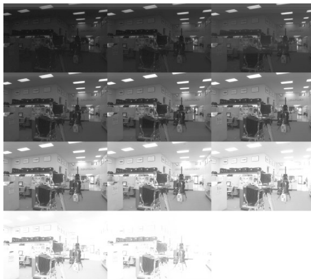
Figure 3: (a) Eleven grayscale photographs of an indoor scene acquired with a Kodak DCS460 digital camera, with shutter speeds progressing in 1-stop increments from \frac{1}{30} of a second to 30 seconds.
