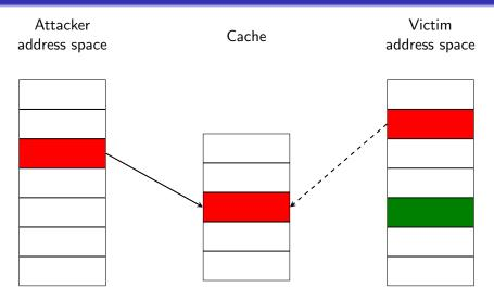
Step 1: attacker loads the encrypt() code into its address space
