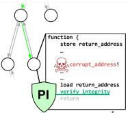
Data pointer integrity is also important (e.g., against data-only attacks and data-oriented programming) and can be (partially) achieved via Pointer Authentication.
