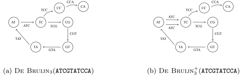
Fig. 7: Comparison of De Bruijn graphs and multigraph of a sample string s = \text{ATCGTATCCA} , for k = 3 . Each vertex represents a unique 2-mer from the string, and each edge represents a unique 3-mer. (a) De Bruijn graph: A walk in the graph corresponds to a substring of s with each k -mer occurring exactly once. (b) De Bruijn multigraph: The edge labels indicate the multiplicity of each 3-mer, thereby allowing the recovery of any substring of s via an appropriate Eulerian path.
