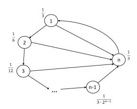
The figure of the graph is shown with the stationary distribution of the ordinary random walk on the graph where every edge has the same weight. In this example, the k-way directed edge conductance is k/n, but the graph has Cheeger constant  $\Omega(1)$  because the vertices  $\{2, 3, ..., n-1\}$  have exponentially decreasing stationary weight.
