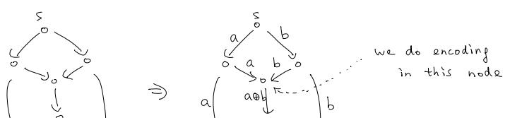
can send two units of information in this example by doing encoding and decoding
