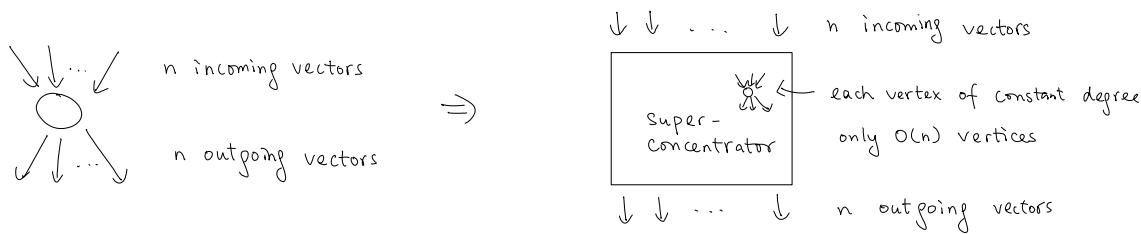
A Superconcentrator is a directed acyclic graph with  $n$  input nodes and  $n$  output nodes, with  $O(n)$  internal nodes each with constant indegree and outdegree.
