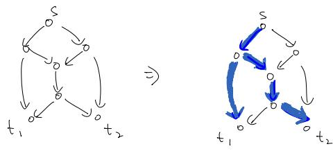
Only one edge-disjoint tree can be found, even though there are two edge-disjoint paths from  $s$  to each  $t_i$ .
