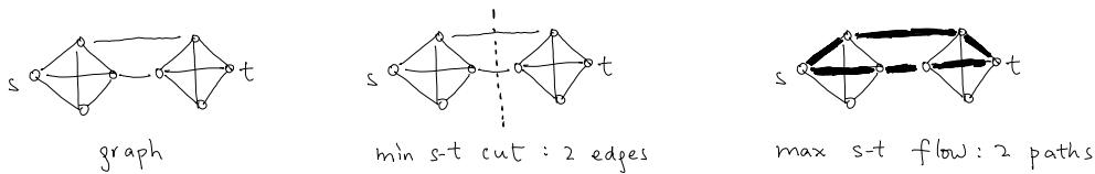
It is not difficult to see that the max  $s$ - $t$  flow value is at most the min  $s$ - $t$  value.
