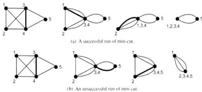
Observation: Each vertex in an intermediate graph is a subset of vertices in the original graph.
