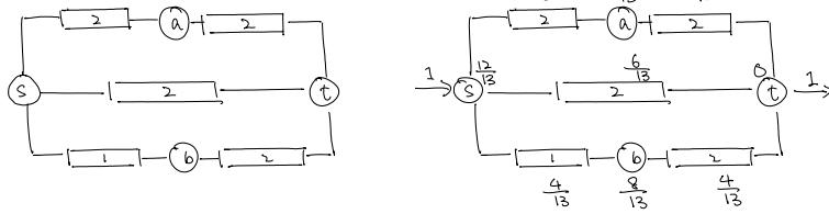
If one ampere is injected into  $s$  and one ampere is removed from  $t$  , then the voltages at the nodes and the currents on the resistors are shown in the figure on the right.
