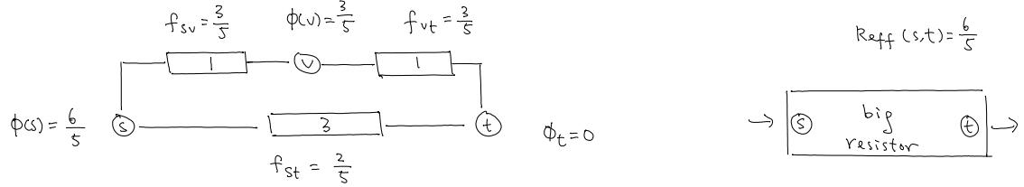
We can think of it as the resistance between  $s$  and  $t$  when the whole network as a single resistor.
