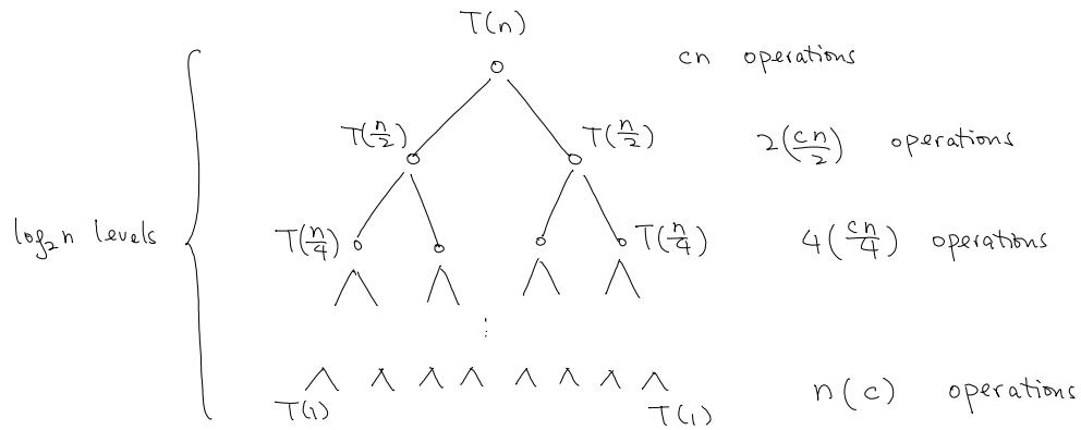
Each level requires  $c_n$  operations, and there are  $\log_2 n$  levels, and so the total time complexity is  $c n \log_2 n$ .
