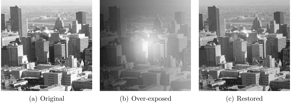
Figure 16: Corruption and restoration of the Montreal image. The total squared error for the over-exposed image is 134,770. The total squared error for the restored image is 13,005 (corresponding to parameter values [163.4 \ 2.047 \ 0.713]^t ).
