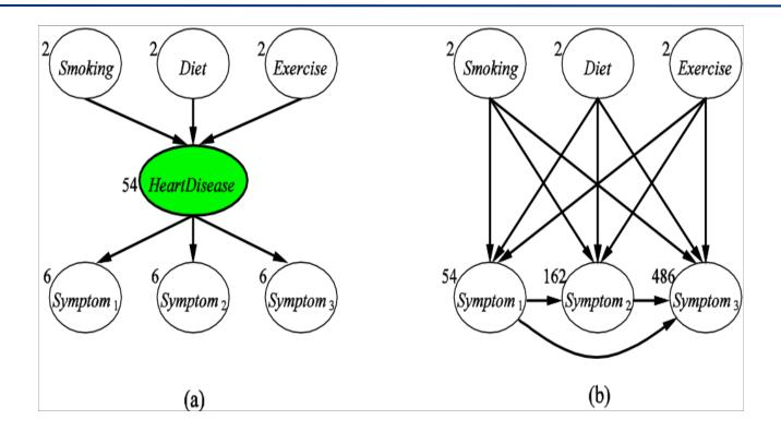
a) Uses a Hidden Variable, simpler (fewer CPT parameters)b) No Hidden Variable, complex (many CPT parameters)
