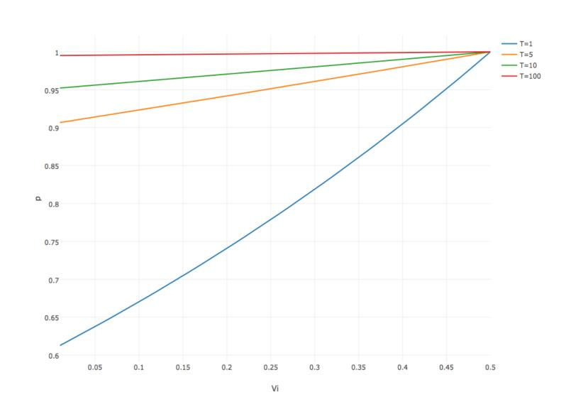
Boltzmann Distribution: T>0 is a parameter called temperature. It starts high and decreases over time towards 0. If T is close to 0 then the prob. of making a bad move is almost 0.
