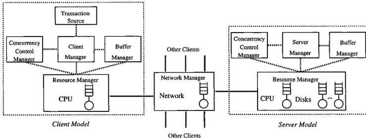
Fig. 4. Performance model of a client-server DBMS.
