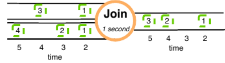
Figure 4: Example illustrating a window operator joining two input streams of SWMs into an output stream of SWMs.
