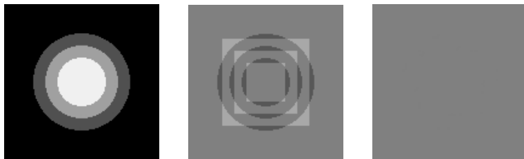
FIGURE 4. Registration results given by the particle model. (Left) deformed template, (middle) difference image between template and target, (right) difference image between deformed template and target.
